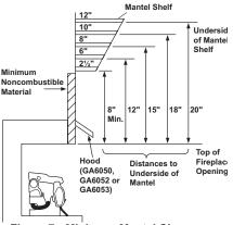
Figure 7 - Minimum Mantel Clearances When Using Hood
